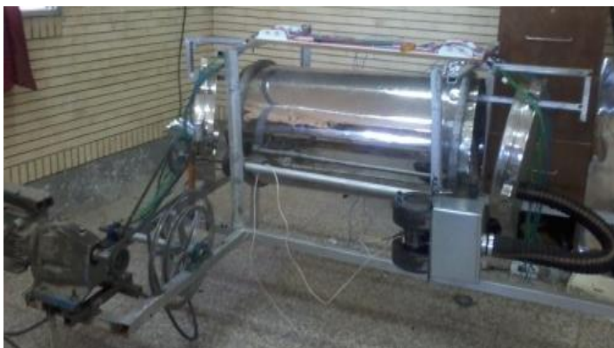
Fig. 1. Optimized apparatus for disinfection of agricultural products
